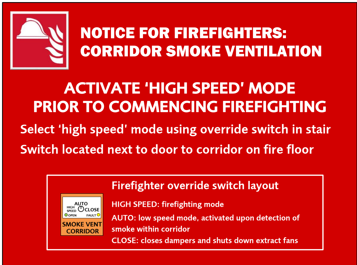
Figure 1: exemplar signage recommended to be provided for firefighters in cases where a variable speed system has been provided. Further information should be provided in the smoke ventilation summary sheet. Type should be 16pt minimum.
