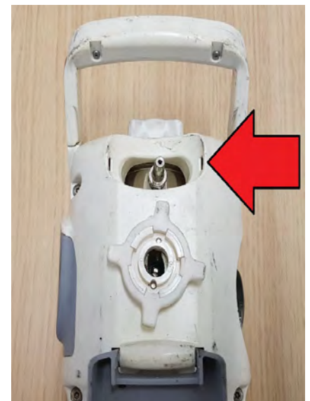
Fig. 2.5 - "Fir tree" connector
