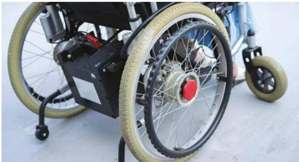
Lithium batteries safely power everyday devices including electric wheelchairs and mobility scooters, but can present a fire risk when overcharged, tampered with, subjected to extremes of temperature (cold or heat), submerged in water or damaged in any way.
