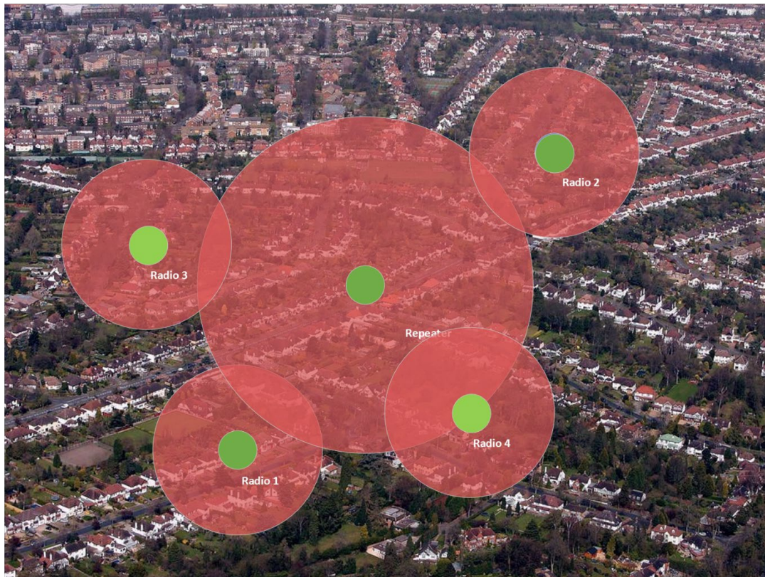
Figure 9 - Repeater positioned centrally between users
