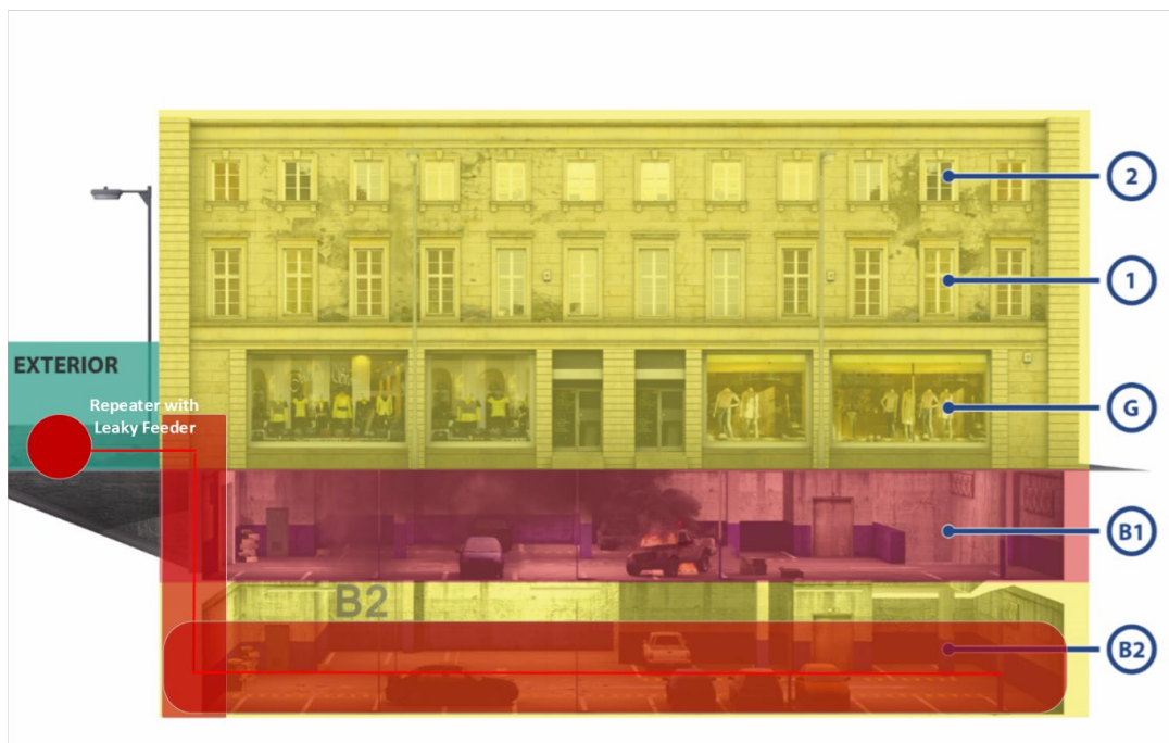
Figure 6 - Image showing leaky feeder deployment and coverage provided
