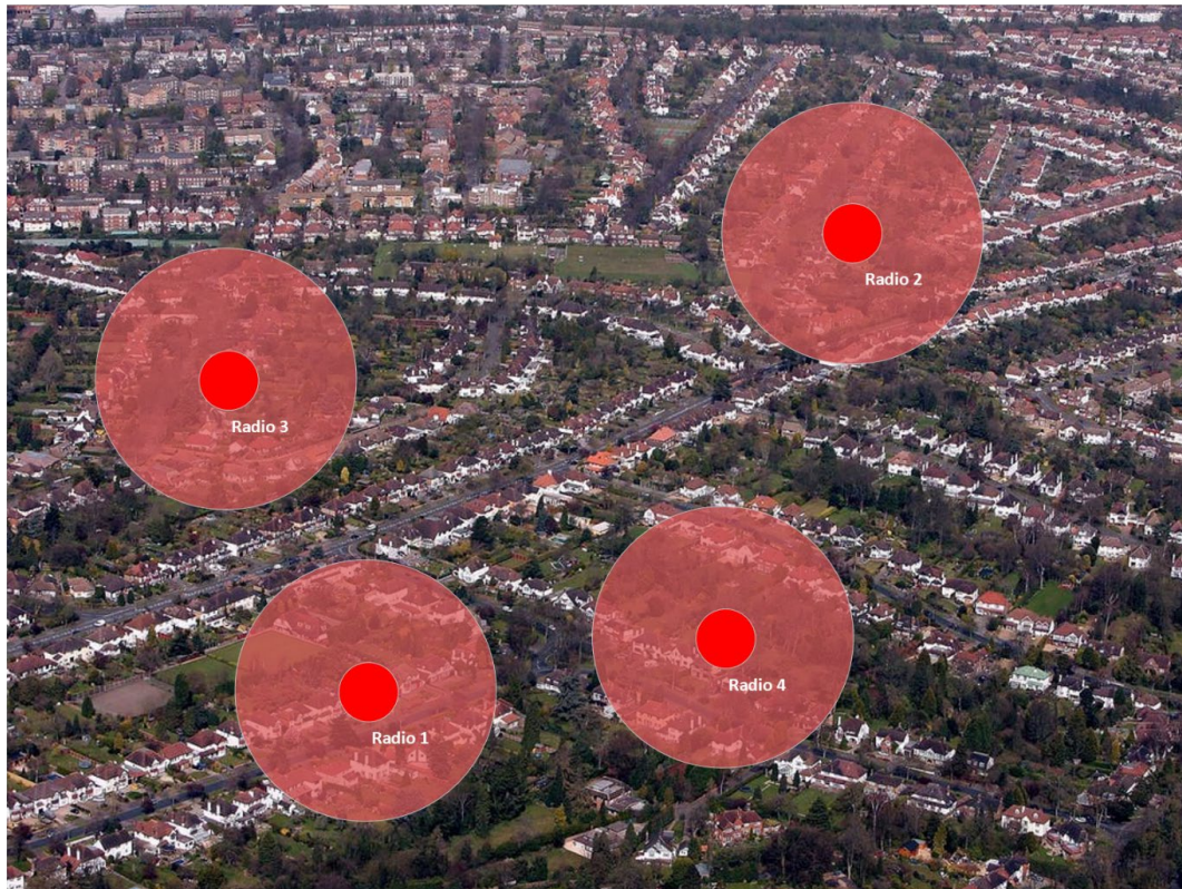
Figure 7 - Radio Coverage without a repeater
