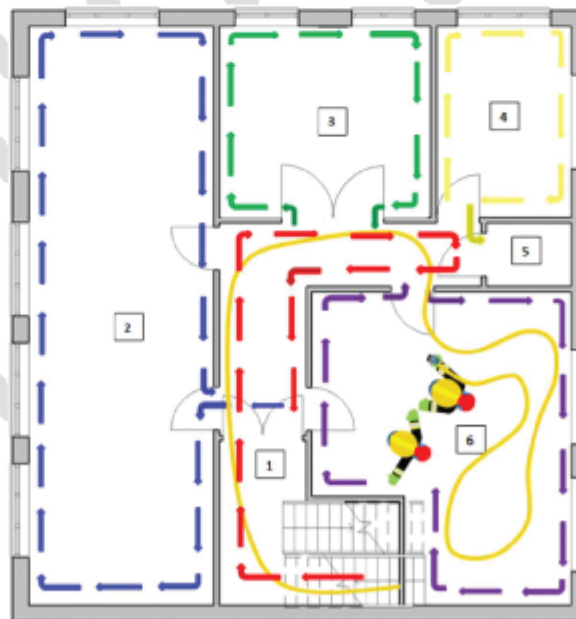
Progressive example of a BA team performing a left hand compartment search.
